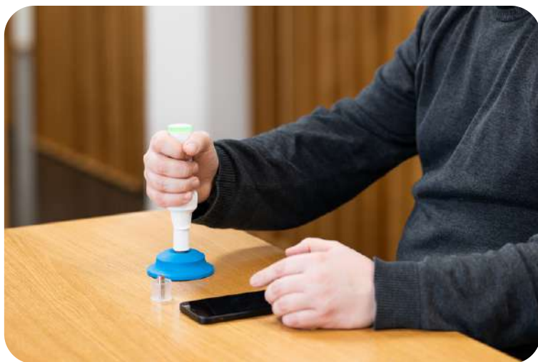
Figure 8: Autoinjector for the automatic administration of a fixed dose of drug
